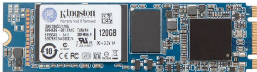
Disco duro M.2 SATA SSD Kingston SSD Now 120GB M.2 SATA SSD. [16]
